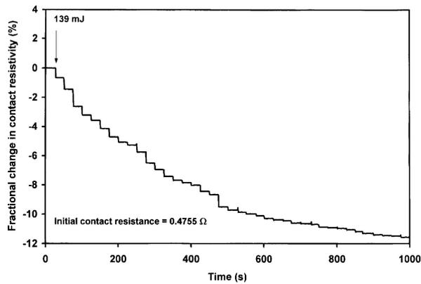
Figure 8 Contact resistance vs. time during repeated impact at an energy of 139 mJ.
