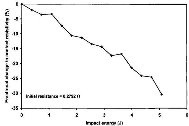
Figure 6 Contact resistance vs. impact energy during impact at progressively increasing energy from 0.36 to 5.08 J.
