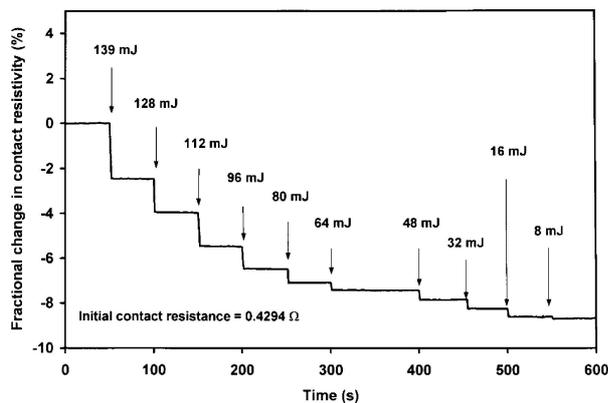
Figure 9 Contact resistance vs. time during impact at progressively decreasing energy from 139 to 8 mJ.
