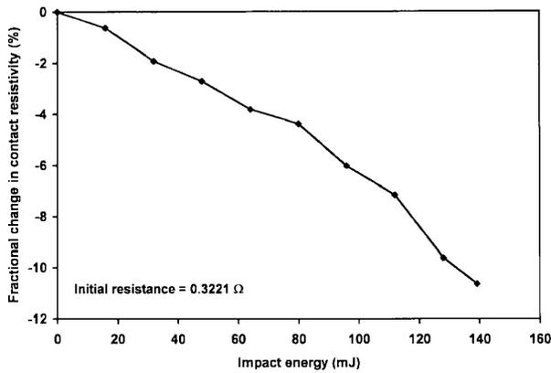
Figure 3 Contact resistance vs. impact energy during impact at progressively increasing energy from 16 to 139 mJ.
