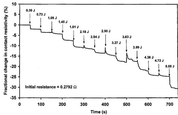
Figure 5 Contact resistance vs. time due to impact at progressively increasing energy from 0.36 to 5.08 J.
