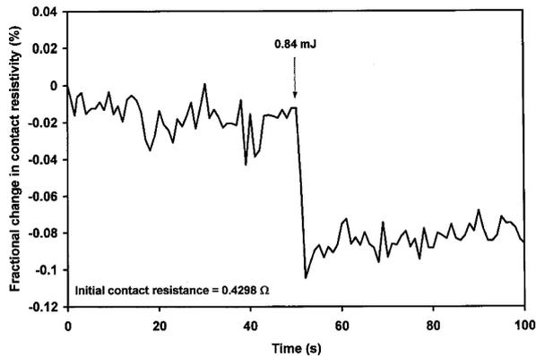
Figure 4 Contact resistance vs. time due to impact at an energy of 0.84 mJ.
