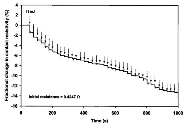
Figure 7 Contact resistance vs. time during repeated impact at an energy of 16 mJ.
