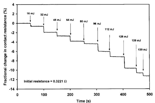
Figure 2 Contact resistance vs. time during impact at progressively increasing energy from 16 to 139 mJ.
