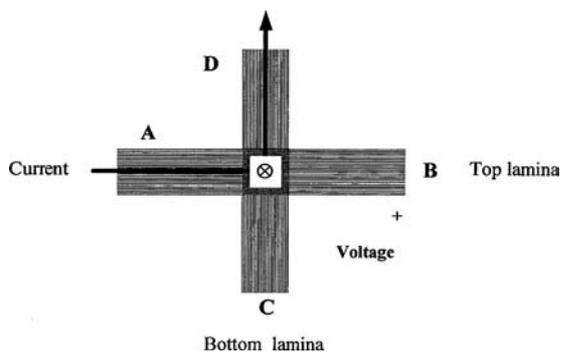
Figure 1 Composite configuration for testing contact resistivity.
